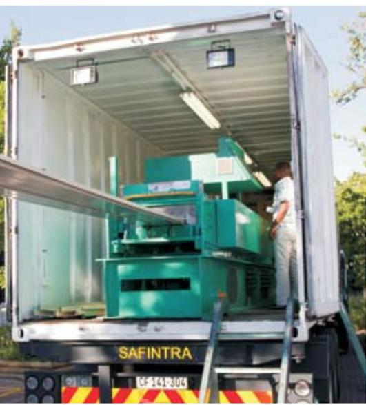
Mobile mills enable Saflok® roof cladding to be rolled on site in continuous lengths of up to 120 metres.
